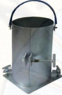
Volumen del molde =  $15\text{cm} \times 30\text{cm} \times H \times D$  →  $5301.438\text{ cm}^3$
