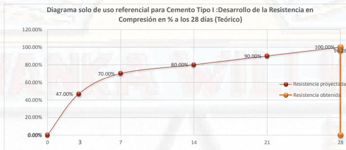
**CURADO CON ICHU STIPA - CONCRETO AUTOCOMPACTANTE F'C = 210 Kg/cm2**
