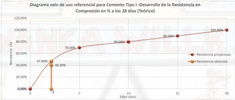
**CURADO CON ASERRÍN- CONCRETO AUTOCOMPACTANTE F'C = 210 Kg/cm2**
