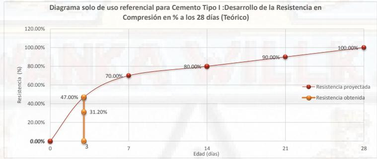
**CURADO CON AISLANTE TÉRMICO- CONCRETO AUTOCOMPACTANTE F'c = 210 Kg/cm2**
