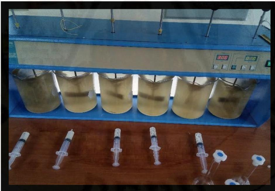
JERINGAS CON DOSIS PARA SER VERTIDOS A CADA VASO TODOS A LA VEZ PARA INICIAR LA MEZCLA RÁPIDA A 300 RPM POR 5 SEGUNDOS
